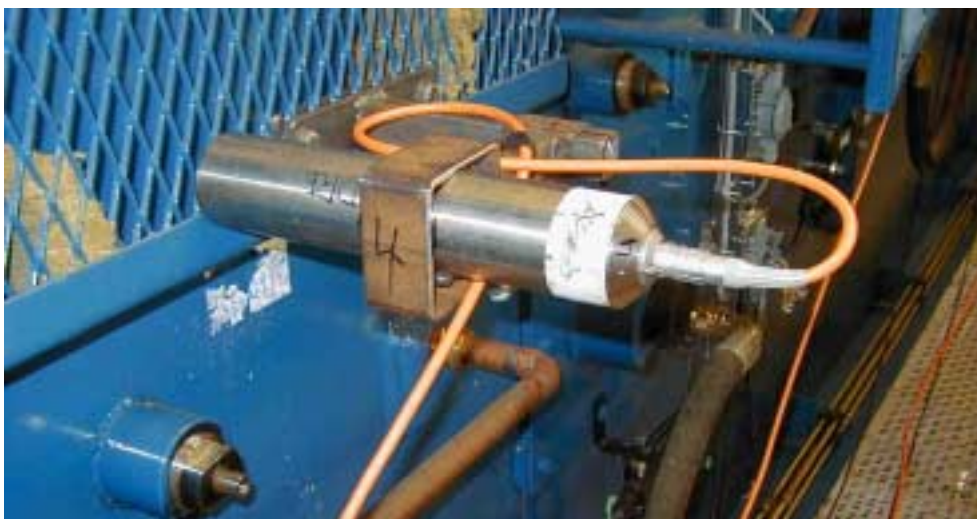
Figur 4: Detektorarrangemang utanpå ugnen. Figure 4: Detector arrangement outside the furnace.
